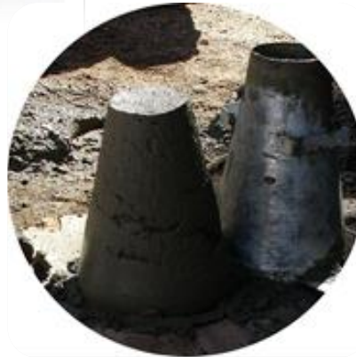
Slump is at 2 ½" with pumpability up to 500' without Plasticizers.
